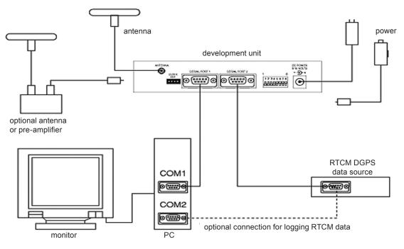
Figure 4-1 Development unit test equipment
